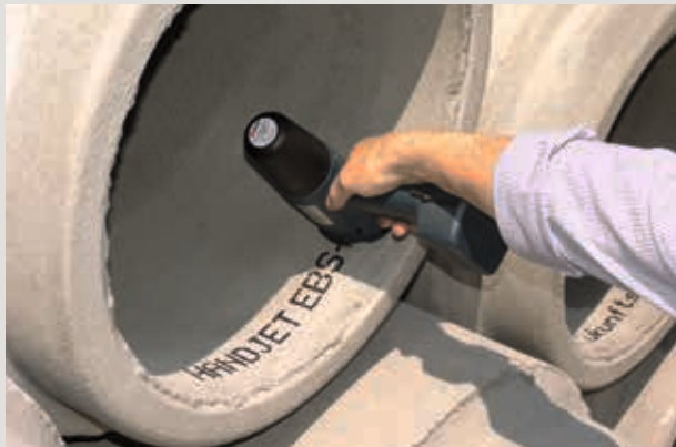
→ Concrete printed with special ink for stronger UV resistance; large spacing wheels.
