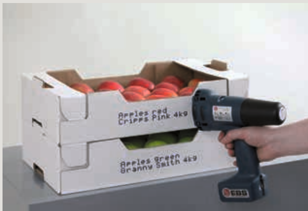
→ Cardboard printed with black universal ink (ethanol).
